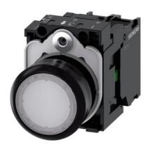
Illuminated pushbutton, 22 mm, round, plastic, white, pushbutton, flat, momentary contact type, with holder, 1NO, LED module with integrated LED 24 V AC/DC, screw terminal, with laser labeling, upper case and lower case, always upper case at beginning of line
