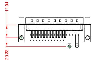
**POWER/CO-AX CONTACT RATING:** (IF PRESENT) SIGNAL CONTACT CURRENT RATING: 5A PER CONTACT SIGNAL CONTACT RESISTANCE:  $10m\Omega$  MAX. **INSULATOR RESISTANCE:**
