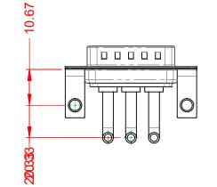
30A (CURRENT) POWER/CO-AX CONTACT RATING: (IF PRESENT) SIGNAL CONTACT CURRENT RATING: 5A PER CONTACT SIGNAL CONTACT RESISTANCE:  $10m\Omega$  MAX. **INSULATOR RESISTANCE:**
