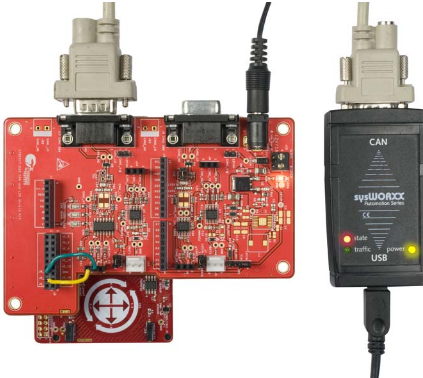
Figure 4-2. CAN Analyzer Connection to CY8CKIT-026's CAN1 Transceiver
