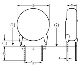
Coating on lead shall not extend below this line.
