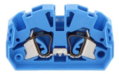
Feed-through terminal for direct mount, Tension-spring connection, Mounting type: Mounting surface, Rated cross-section: 2.5 mm<sup>2</sup>, Width: 11.1 mm, Colour: Blue
