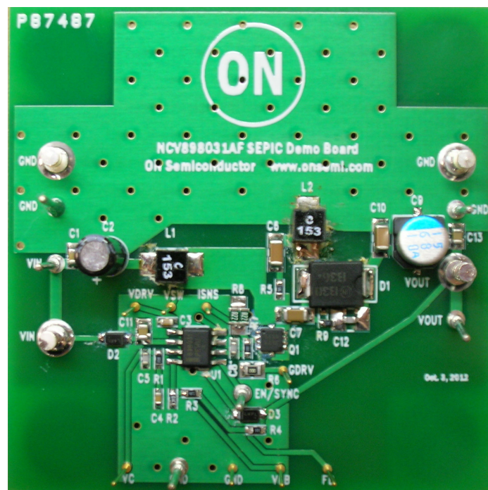
Figure 1. NCV898031 SEPIC Evaluation Board
