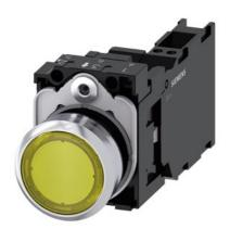
Illuminated pushbutton, 22 mm, round, metal, shiny, yellow, pushbutton, flat, momentary contact type, with holder, 1 NO+1 NC, LED module with integrated LED 24 V AC/DC, spring-type terminal, with laser labeling, upper case
