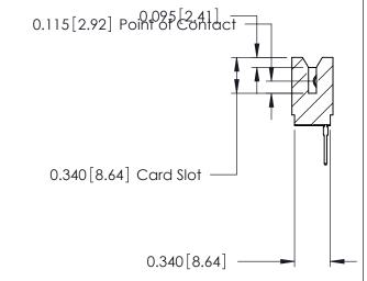
ACAD REFERENCE NO. 746 Series Ultra-Mate Card Edge Connector - Press Fit DRAWN: Part Number: 746-036-527-506 CHECKED: **EDAC INC** SCALE: THESE DRAWINGS AND SPECIFICATIONS ARE THE PROPERTY OF EDAC INC.,AND TORONTO, ONTARIO SHALL NOT BE REPRODUCED, OR COPIED CANADA OR USED AS THE BASIS FOR THE MANUFACTURE OR SALE OF APPARATUS
