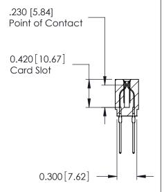
ACAD REFERENCE NO. 725 Series Ultra-Mate Card Edge Connector - Press Fit DRAWN: Part Number: 725-046-545-201 CHECKED: **EDAC INC** THESE DRAWINGS AND SPECIFICATIONS
