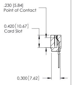
ACAD REFERENCE NO. 725-ENG MASTER 725 Series Ultra-Mate Card Edge Connector - Press Fit SEGAHON:3A:9A DRAWN: J.LEE Part Number: 725-024-545-101 CHECKED: DATE: SCALE: **EDAC INC** SHEET 1 OF 1 THESE DRAWINGS AND SPECIFICATIONS ARE THE PROPERTY OF EDAC INC.,AND TORONTO, ONTARIO SHALL NOT BE REPRODUCED, OR COPIED DRAWING NUMBER **ISSUE** CANADA OR USED AS THE BASIS FOR THE 725-ENG MASTER MANUFACTURE OR SALE OF APPARATUS YOUR CONNECTION TO QUALITY & SERVICE WITHOUT WRITTEN PERMISSION.
