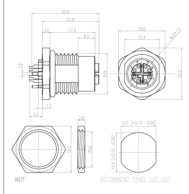
NOTE: MATERIAL HOUSING: PA66 UL94V-0, BLACK CONTACT: **BRASS** NUT: **BRASS** SHELL: **BRASS** □-RING: EPDM, BLACK ZINC ALLOY X-SHELL: **FINISH** CONTACT: GOLD 104" MIN. □VER 504" NICKEL NUT: NICKEL PLATED SHELL: NICKEL PLATED X-SHELL: NICKEL PLATED **ELECTRICAL** RATED CURRENT: 0.5A RATED VOLTAGE: 50VAC/60VDC INSULATION RESISTANCE: 100 MOhms MIN. CONTACT RESISTANCE: 10 mDhms MAX. WATER PROOF: IP67 **ENVIRONMENT OPERATION TEMPERATURE:** -40°C TD +85°C MAX WIRE AWG: 24
