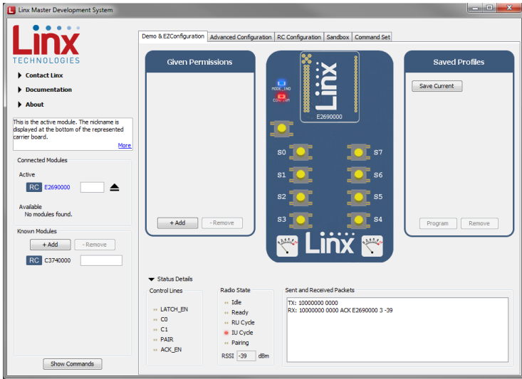
Figure 31: The Master Development System Software Transmitting Module
