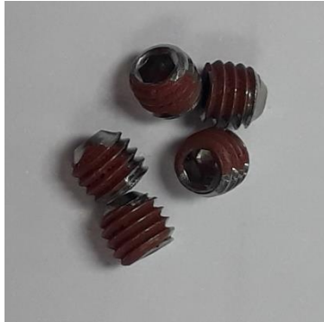
Photo#2- Set screw with Loctite coating
