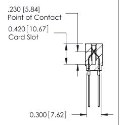
725 Series Ultra-Mate Card Edge Connector - Press Fit ACAD REFERENCE NO. Part Number: 725-044-541-201
