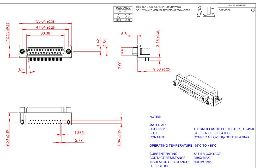
WITHSTANDING VOLTAGE: 1000V AC rms
