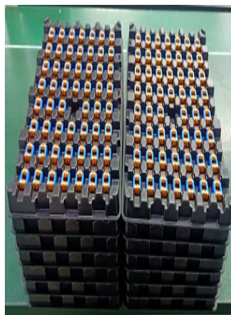
Picture 2: New package Blister tray in cardboard box
