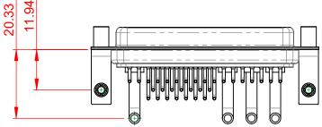
**OPERATING TEMPERATURE:** POWER/CO-AX CONTACT RATING: 30A (CURRENT) (IF PRESENT) SIGNAL CONTACT CURRENT RATING: 5A PER CONTACT SIGNAL CONTACT RESISTANCE:  $10m\Omega$  MAX.
