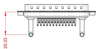
40A (CURRENT) POWER/CO-AX CONTACT RATING: (IF PRESENT) SIGNAL CONTACT CURRENT RATING: 5A PER CONTACT SIGNAL CONTACT RESISTANCE:  $10m\Omega$  MAX. **INSULATOR RESISTANCE:** 5000MΩ min. DIELECTRIC
