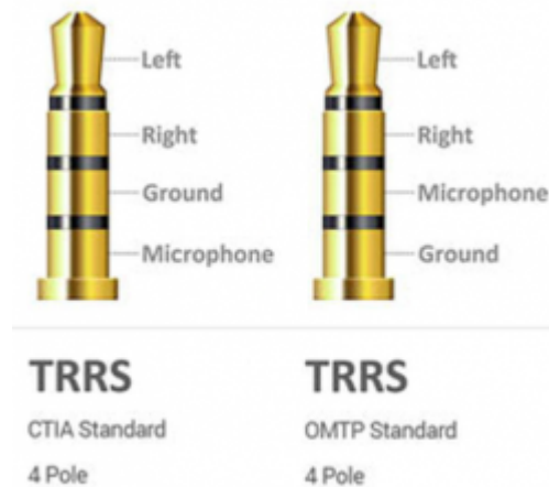
Two of the more common variations of the headphone jack connection standards. (Click to enlarge) Source: quora.com
