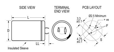
**General Information** Series ALC70 Dielectric Aluminum Electrolytic Description Snap-In, Aluminum Electrolytic RoHS Lead 3 Pin Short AEC-Q200 No Halogen Free Yes 105 g Component Weight Notes Dimensions D And L Include Sleeving. Shelf Life 156 Weeks
