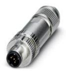
Bus system connector, PROFIBUS DP (12 Mbps), 3-position, shielded, Plug straight M12, B-coded, Push-in connection, knurl material: Zinc die-cast, nickel-plated, external cable diameter 4 mm ... 8 mm
