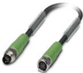
Sensor/actuator cable, 4-position, PUR halogen-free, black-gray RAL 7021, shielded, Plug straight M8, on Socket straight M8, cable length: 0.6 m
