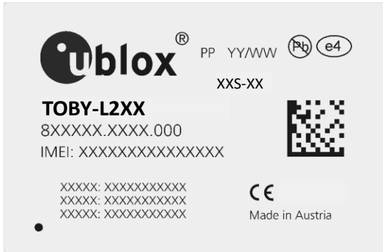
Figure 7: Example of TOBY-L2 series module label
