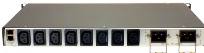
Figure 3-9 200-240 VAC SLB - Branch Office Manager Power Outlets
