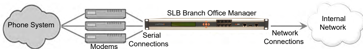
Figure 10-2 Remote Access Server
