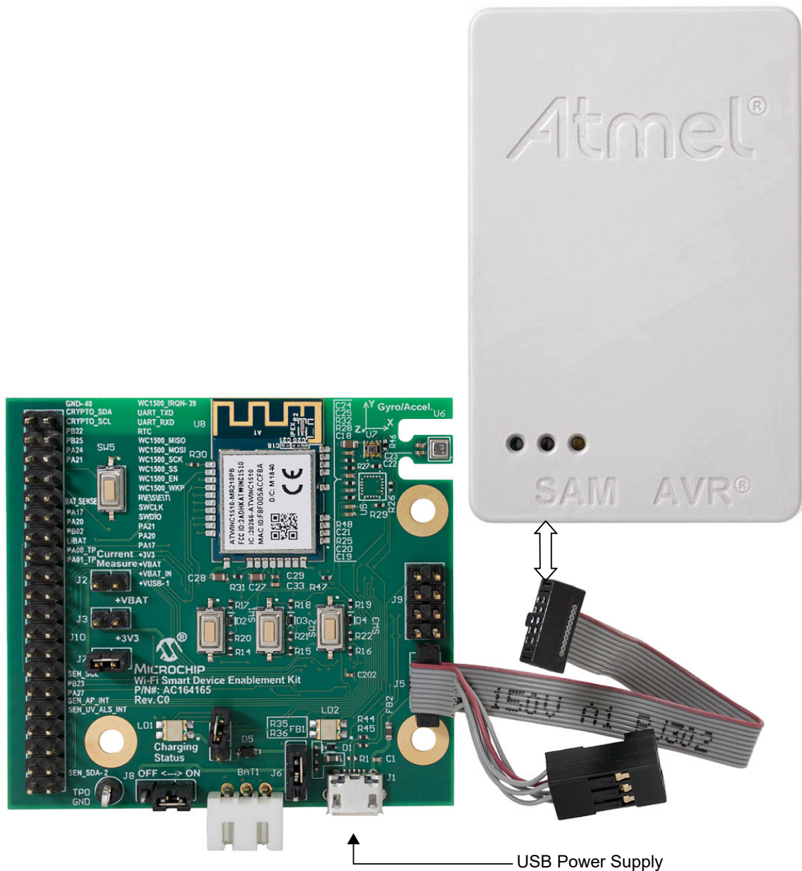
Figure 4-3. Atmel ACE Connected to Board
