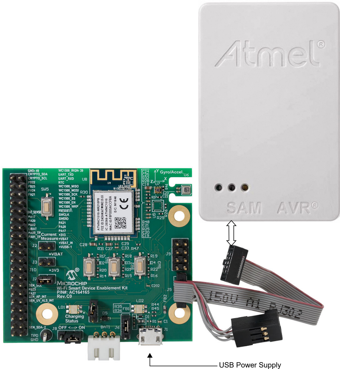
Figure 3-2. Atmel ICE Connected to the Board SWD Interface Connector (J5)
