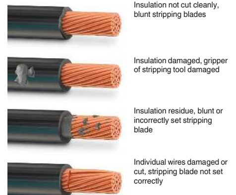
Cable stripped incorrectly according to DIN IEC 60352
