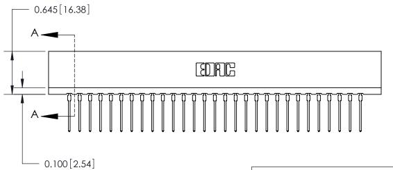
737 Series Ultra-Mate Card Edge Connector - Press Fit
