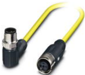
Sensor/actuator cable, 3-position, PVC, yellow, shielded, Plug angled M12 SPEEDCON, A-coded, on Socket straight M12 SPEEDCON, A-coded, cable length: 1.5 m
