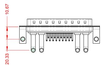
POWER/CO-AX CONTACT RATING:40A (CURRENT)(IF PRESENT)SIGNAL CONTACT CURRENT RATING:5A PER CONTACTSIGNAL CONTACT RESISTANCE:10mΩ MAX.INSULATOR RESISTANCE:5000MΩ min.DIELECTRIC5000MΩ min.
