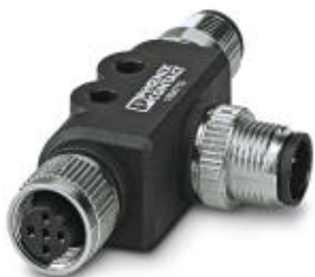
T distributor, PROFIBUS DP (12 Mbps), 5-position, shielded, Socket straight M12, B-coded, on Plug straight M12, B-coded and Plug straight M12, B-coded, Thread M12 plug input not rotatable
