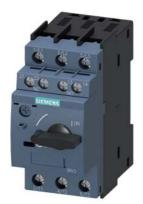
Circuit breaker size S0 for motor protection, CLASS 10 A-release 5.5...8 A N-release 104 A screw terminal Standard switching capacity with transverse auxiliary switches 1 NO+1 NC
