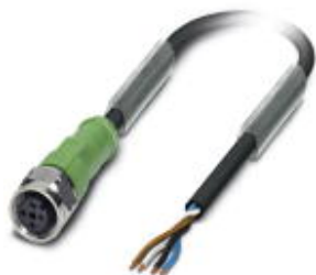
Sensor/actuator cable, 4-position, PUR halogen-free, black-gray RAL 7021, free cable end, on Socket straight M12, A-coded, cable length: 10 m
