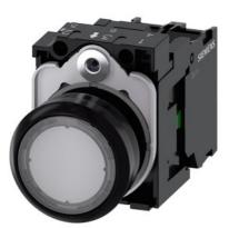
Illuminated pushbutton, 22 mm, round, plastic, clear, pushbutton, flat, momentary contact type, with holder, 1NO, LED module with integrated LED 110 V AC, screw terminal, with laser labeling, inscription or symbol Customer-specific selection with SIRIUS ACT configurator (CIN)
