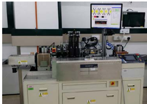
Current Automatic Vision only top inspection
