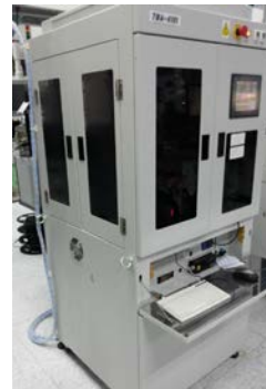
Glass Turret- top, bottom and side inspection possible
