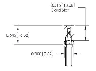
ACAD REFERENCE NO. 737 Series Ultra-Mate Card Edge Connector - Press Fit DRAWN: Part Number: 737-030-541-201 CHECKED: **EDAC INC** SCALE: THESE DRAWINGS AND SPECIFICATIONS ARE THE PROPERTY OF EDAC INC.,AND TORONTO, ONTARIO SHALL NOT BE REPRODUCED, OR COPIED DRAWING NUMBER CANADA OR USED AS THE BASIS FOR THE MANUFACTURE OR SALE OF APPARATUS YOUR CONNECTION TO QUALITY & SERVICE WITHOUT WRITTEN PERMISSION.
