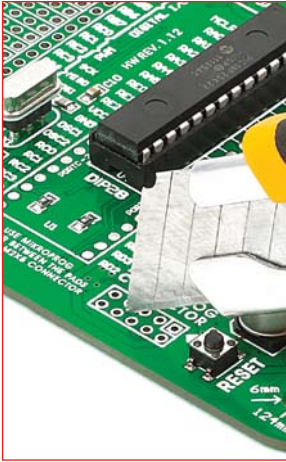
Figure 3-2: cutting copper between pads for the external programmer
