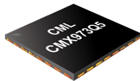
32-pin VQFN (5mm x 5mm x 1mm)
