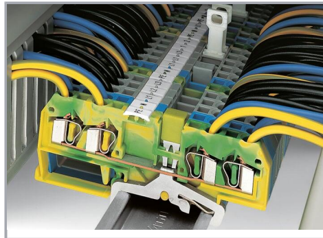
Steel DIN-rails are not suited for PEN (ground and N-conductor) applications per EN 60947-7-2 (VDE 0611, Part 3).
