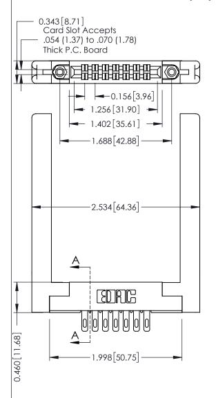
Point of Contact 305 / 315 / 355 Card Edge Connector J.LEE Part Number: 355-014-500-258 NTS 305 Assembly
