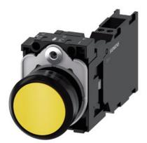
Pushbutton, 22 mm, round, plastic, yellow, pushbutton, flat, momentary contact type, with holder 1 NO+1 NC, spring-type terminal, with laser labeling, inscription or symbol Customer-specific selection with SIRIUS ACT configurator (CIN)
