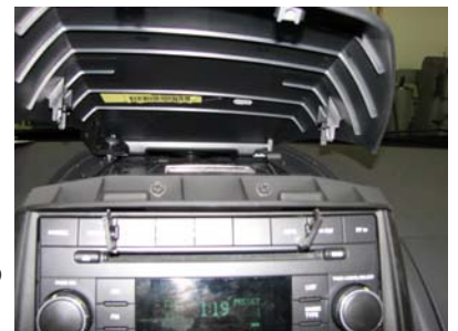
Cover Removal and screws under cover
