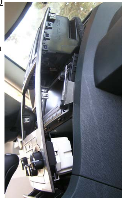
Bezel removed picture
