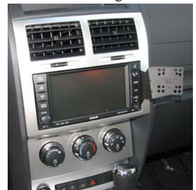
Install Picture of InDash on Dodge Nitro
