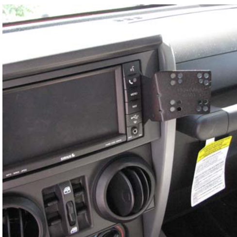
InDash Mount in place showing location
