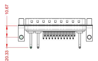
POWER/CO-AX CONTACT RATING:10A (CURRENT)(IF PRESENT)SIGNAL CONTACT CURRENT RATING:5A PER CONTACTSIGNAL CONTACT RESISTANCE:10mΩ MAX.INSULATOR RESISTANCE:5000MΩ min.DIELECTRIC5000MΩ min.
