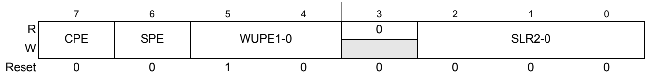
Figure 21-3. CAN Physical Layer Control Register (CPCR)
