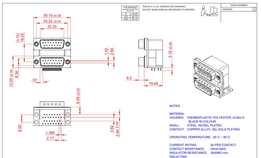
WITHSTANDING VOLTAGE: 1000V AC rms
