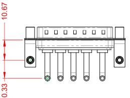
POWER/CO-AX CONTACT RATING: (IF PRESENT) SIGNAL CONTACT CURRENT RATING: 5A PER CONTACT SIGNAL CONTACT RESISTANCE:  $10m\Omega$  MAX.
