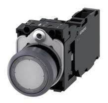
Illuminated pushbutton, 22 mm, round, plastic with metal front ring, clear, pushbutton, flat, momentary contact type, with holder, 1 NO+1 NC, LED module with integrated LED 110 V AC, screw terminal, with laser labeling, inscription or symbol Customer-specific selection with SIRIUS ACT configurator (CIN)
