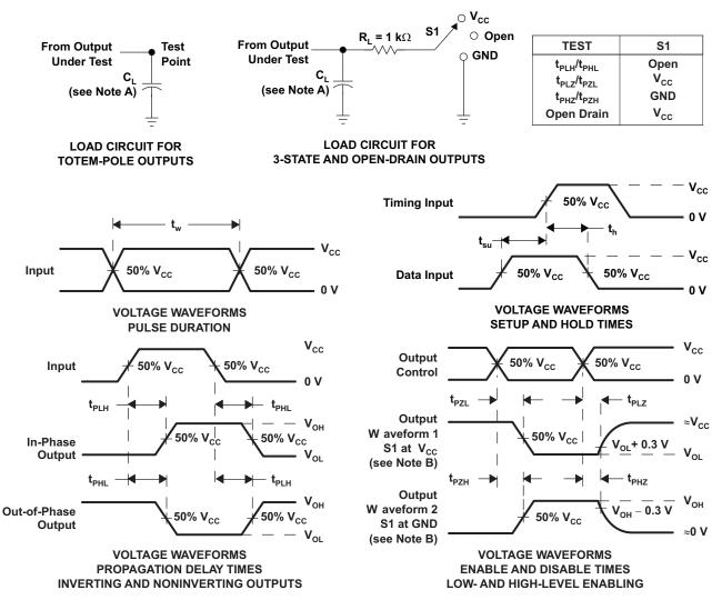
**NOTES:** A. C<sub>1</sub> includes probe and jig capacitance.
