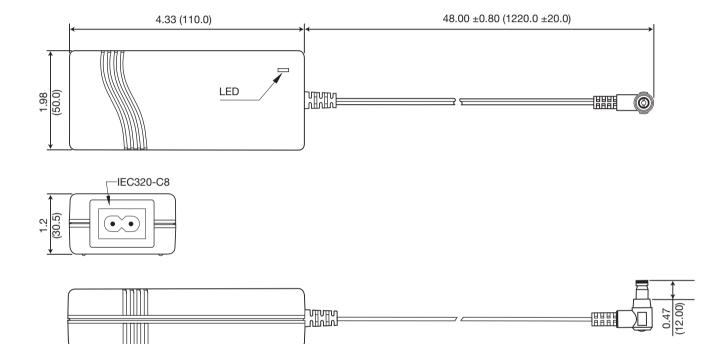
Output connector is right angle jack 0.22  $\times$  0.10  $\times$  0.47 (5.5  $\times$  2.5  $\times$  12.0), center postive. Weight: 0.49 lbs (220 g). Case tolerance:  $\pm$ 0.02 ( $\pm$ 0.5) All dimensions in inches (mm).
