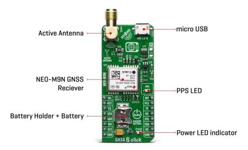
Note: Button battery 1.55V is provided with the GNSS 7 click
